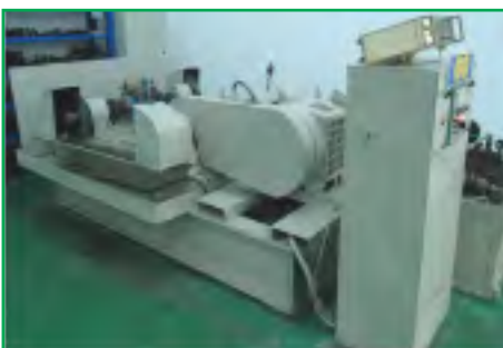
Test di usura Chain wear testing machine
