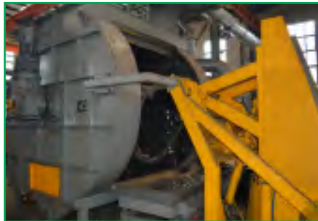
Trattamento pallinatura lamiera-Incremento resistenza a fatica Plate strong shot peening treatment-improve fatigue strength
