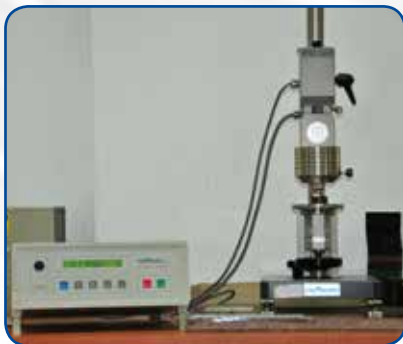
Durometro Micro hardness tester
